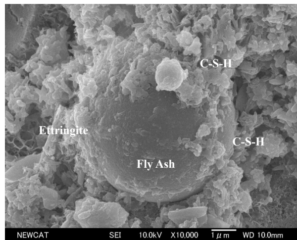
Photo 4 SEM Photo of [3h Steam(80℃) Cured] Non-Burnt Brick Specimen (FA:India-A) (×10000)
