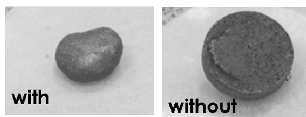
Fig. 11 Comparison between with and without ash treatment of "Oak Bark" at 1350 °C: 10 min
