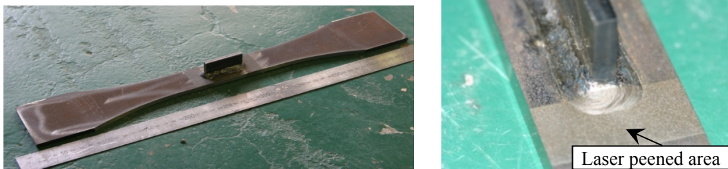
Fig.9 Photo of box-welded rib specimen and its laser peening area
