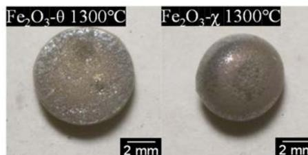
Fig. 11 Appearances of  $\text{Fe}_2\text{O}_3\text{-}\theta$  and  $\text{Fe}_2\text{O}_3\text{-}\chi$  before and after heated up to  $1300^\circ\text{C}$
