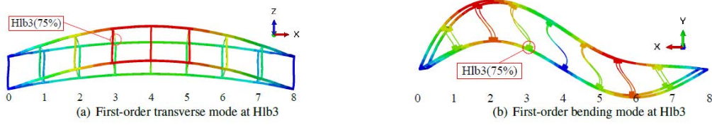
Figure 5 Natural vibration modes at single damage
