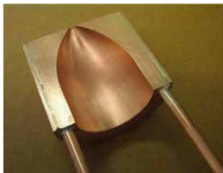
Figure 8: Photograph of concentrator for molten Si jet.
