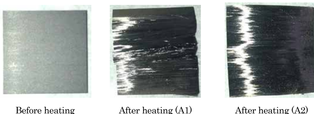
Fig. 6 Appearance of samples after microwave heating (sample 2)
