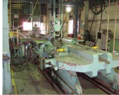
Fig. 1 Ten MN tension testing machine used for wide plate tests
