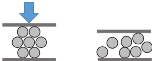
Fig.8 Increase of voids in cluster particle when large deformation
