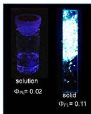
Figure 3. Photographs of 4 in THF ( $1 \times 10^{-5}$  M) and solid state under UV-irradiation.
