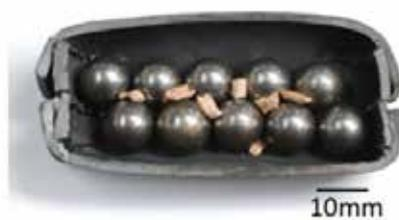
**Fig.4** Appearance view of SUS balls and biomass on SUS boat.
