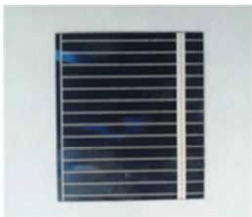
Fig.8 Solar cell before etching
