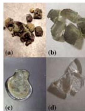
Fig.2 Appearance of intermediates synthesized from various raw materials ( (a) from fly ash, R = 0.5 , (b) from fly ash, R = 1.0 , (c) from bone powder, R = 1.0 , and (d) from \text{CaCO}_3 reagent, R = 1.0 )
