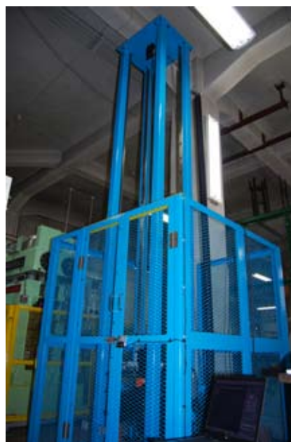
Fig.2 Drop-weight test machine
