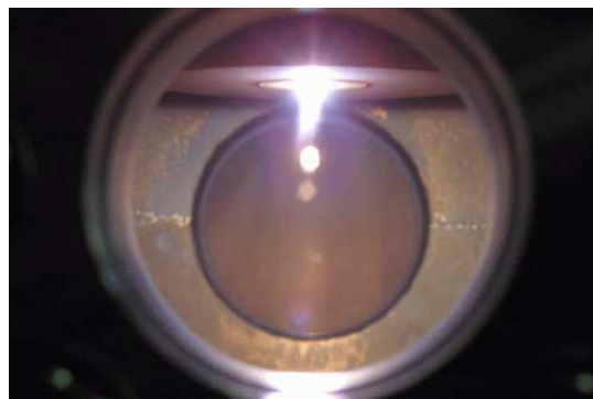
Fig.9 Direct photograph of O 2 PJ in O 2 atmosphere (P = 0.5 MPa)
