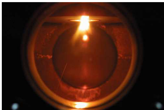
Fig.8 Direct photograph of O 2 PJ in N 2 atmosphere (P = 0.5 MPa)
