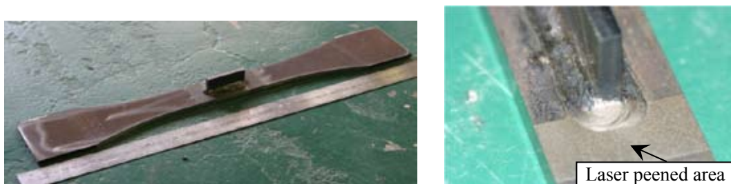
Fig.9 Photograph of a box-welded rib specimen and its laser-peened area
